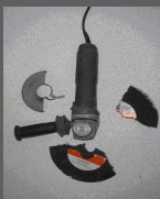
Angle grinder and disintegrated disk
